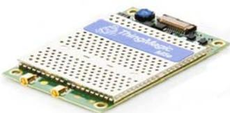
The 2-port M5e is designed for adding UHF RFID read/write capabilities to a wide range of products and solutions, from high-speed label printing and inlay testing, to stationary, mobile, and handheld computers. The M5e will transmit up to +30 dBm.
