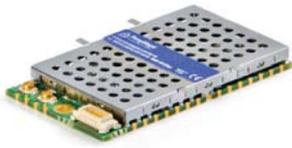
This module is designed to meet the demands of high performance RFID handheld, mobile, and stationary readers. The Micro offers two antenna ports and supports the ability to transmit up to +30 dBm for demanding applications. The edge connections for signals, power, and RF allow the module to be soldered directly to a motherboard as a standard component. The on-board connectors allow the module to be mated to a motherboard as an add-on option.
